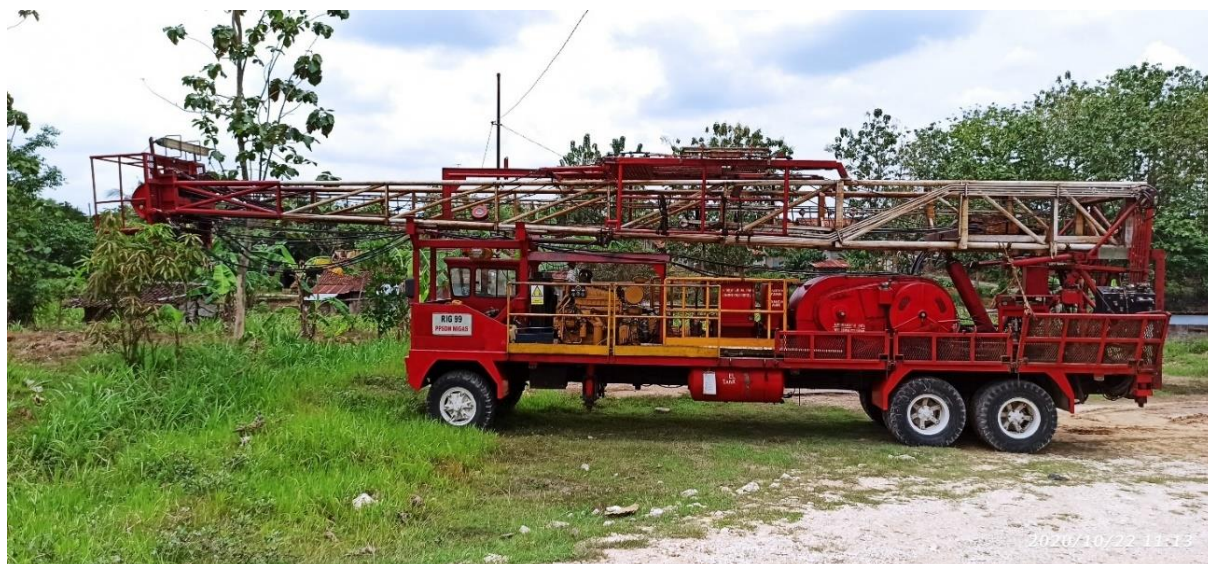
Figure 4. Rig down and be ready for moving
